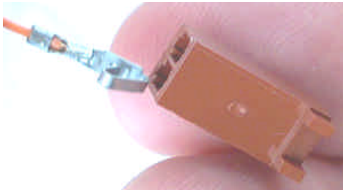
Figure 7: Correct Reset Pin Orientation and Location During Insertion into the Connector Housing
